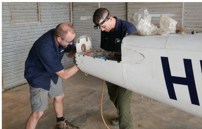
Jason and I removed the tail of HR-AUS to replace a cracked stabilizer bracket. In this photo we are riveting the bracket in place.
